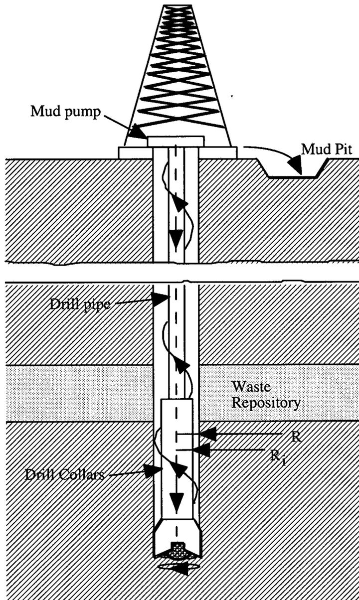
Figure 3. Detail of rotary drill string adjacent to repository.
