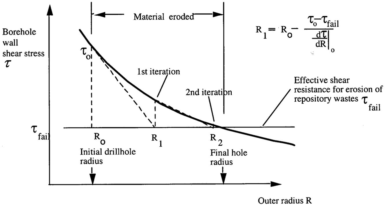
Figure 4. Iterate to find the final hole radius
