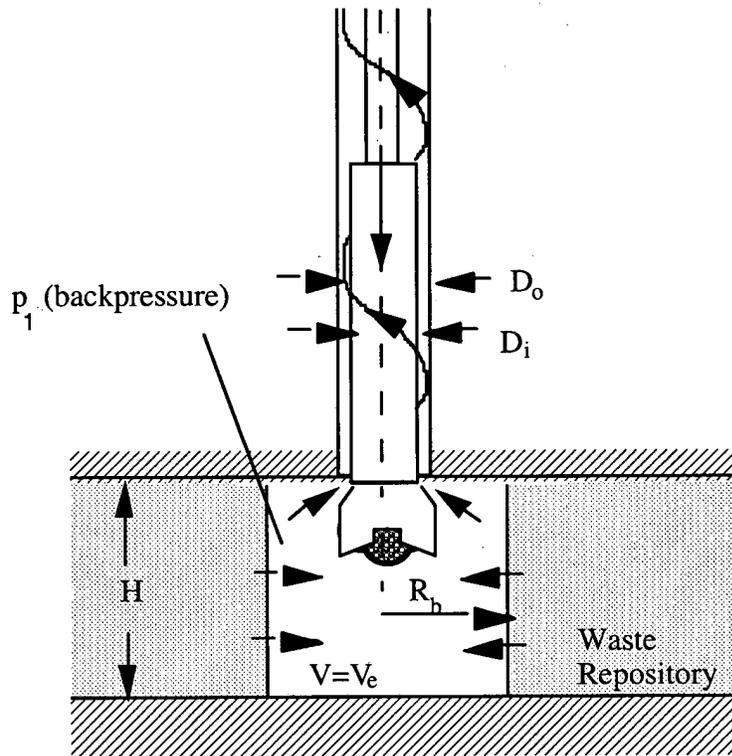
Figure 6 Idealized Cylindrical Final Volume Release Configuration
