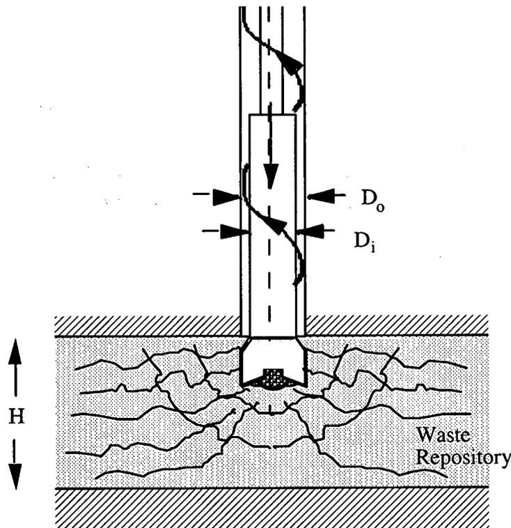
Figure 7 Fractured Waste Matrix after Penetration
